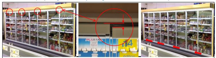
It may be necessary to slide all lower profiles in one or in the other direction to be able to adjust the level of the doors. If the sliding of the frames does not allow a perfect adjustement, make an average adjustment that can be refined later.
